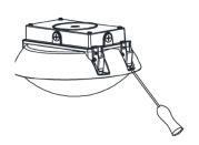
1. Pry open the spring buckle using a suitable screwdriver.
