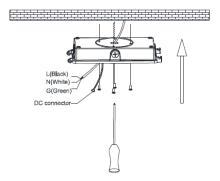
4. Lock the back plate to the wall or J-box by a suitable screwdriver.
