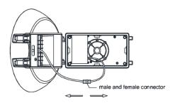
2. Unplug the male and female connectors, and then seperate lampbody from the back plate.
