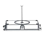
3. Take down 1/2" screw from the back plate by a suitable screwdriver.
