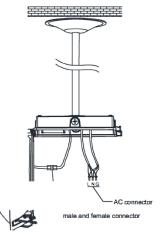
5. Use the hinge to lock the lampbody to the back plate firmly, and then connect the main power. Connect the male and female connectors together.
