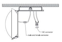
5. Use the hinge to lock the lampbody to the back plate firmly, and then connect the main power. Connect the male and female connectors together.
