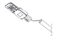
2. Loosen the monting screws on the pole sleeve.
