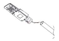
1. Connect the wires to AC input power correctly.
